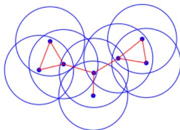
**Figure:** The corresponding unit disk graph
